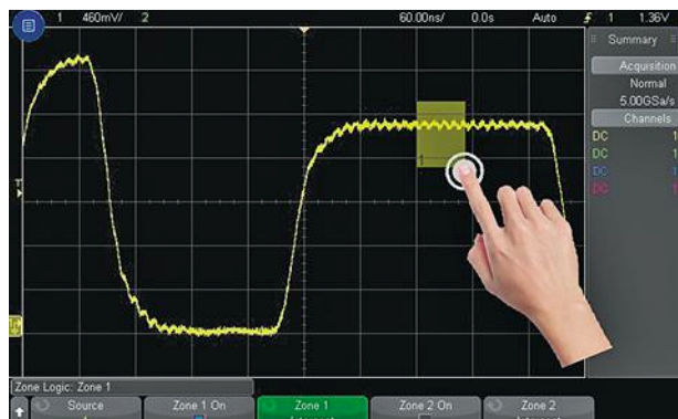
3. "Zone triggering" on a touchscreen scope simplifies runt trigger setup, which in this case is on the widest positive runt.
